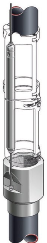
PCP Gauge with clamp-on gauge carrier & ported collar
